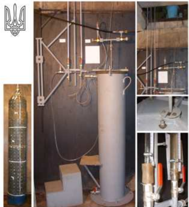
Fig. 2. Block-diagram and photo of “water jacket” unit implemented at the E. O. Paton Institute for cylinder testing for permanent expansion. (A B are burettes).
